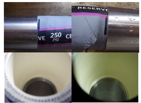
Final permanent stretch E1/E2 = .03" Inner tube seal to fitting end looks good
