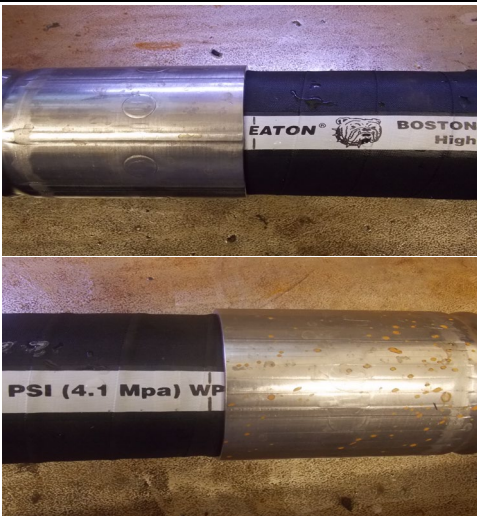
E1 and E2 Pre-Failure, taken around 3000 psi
