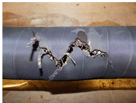
Hose burst-Failure at 3539 psi
