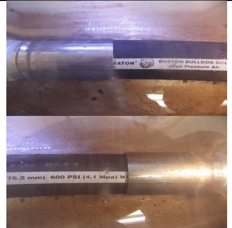
E1 and E2 after heat soak, prior to pressurization
