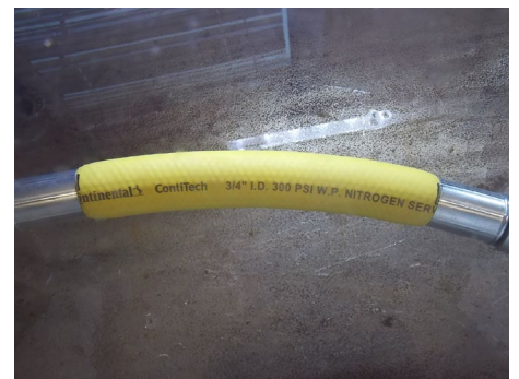
Photo taken at 1254 psi, prior to burst
